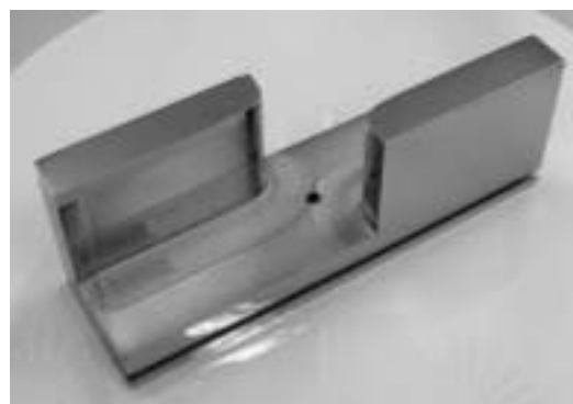
Fig. 6. Channel cut Si(311) crystal for a fixed exit beam. Total length 100 mm, reflecting surfaces 45 mm.
