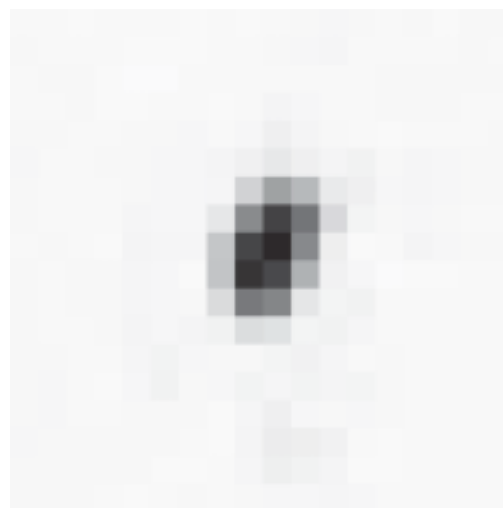
Fig. 3. A 2D scan of \Delta\mu_x of the sample with the focused X-ray beam. The dark area is about 50 \mu\text{m} in horizontal width and has about half the thickness of the surrounding region due to an accumulated ablation of the sample at a higher laser intensity than used in the measurements reported here.
